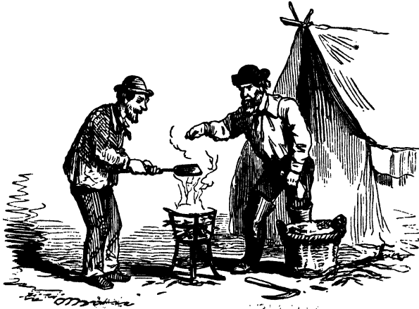
Fig. 116. Testing for Pyrites by the red-hot Shovel.
